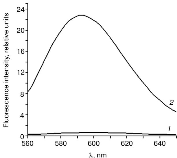
**Fig. 6.** Fluorescence spectra with light ( $\lambda = 540$  nm) excitation of: 1) ethidium bromide (2.2  $\mu\text{M}$ ); 2)  $\lambda$  phage DNA (5.5  $\mu\text{M}$ )–ethidium bromide (2.2  $\mu\text{M}$ ) complex.
